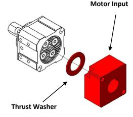
**Step 5**: Be sure to add a pea-sized amount of included Red Tacky Grease (am-2768) to the gear teeth. If more than one stage is present, add grease to each stage.
