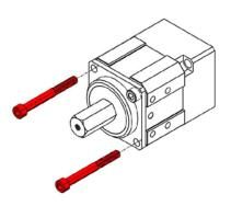
**Step 4**: Attach the Motor Input Block to the CIM Motor (with previously attached pinion) using the included 10-32x1250 Socket Head Screws. Be sure to install the Motor Input Block with the flat side against the motor.
