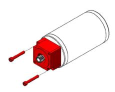
**Step 6**: Reinstall the Thrust Washer into the CIM Sport onto the surface of the gears inside the gearbox. Insert the Motor Assembly into the gearbox, and gently turn the output shaft until the gears mesh.
